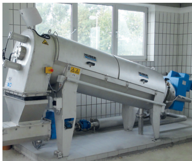
Stationary mounted screw press for 140 kgDS/h
