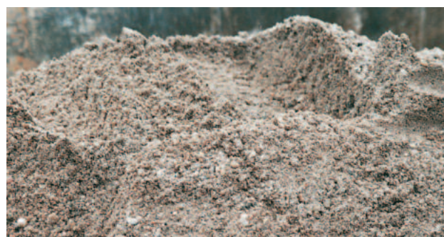
Washed grit of a wastewater treatment plant
