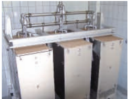
Modular design – installation with 6 modules, 84 m 2 membrane area
