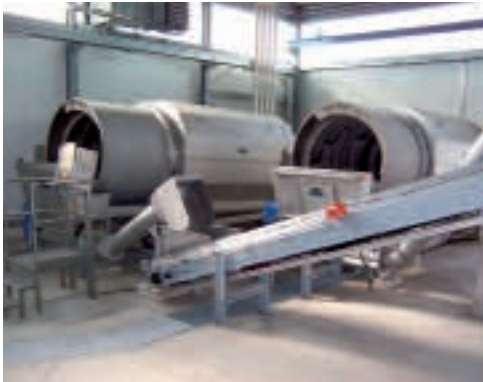
Washing of contaminated grit with the versatile ROTAMAT® Wash Drum RoSF 9
