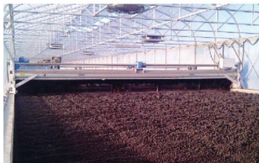
Dewatered sewage sludge becomes dry granulate with the SRT system
