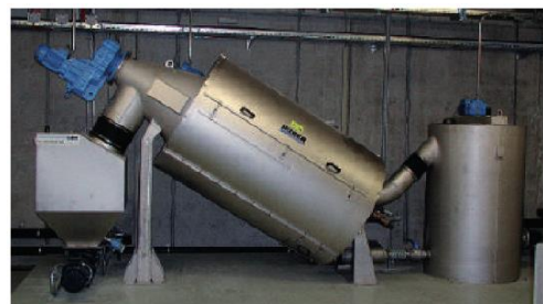
Extremely sturdy: HUBER Rotary Screw Thickener S-DRUM
