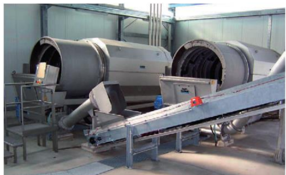
Washing of contaminated grit with the versatile HUBER Wash Drum RoSF9
