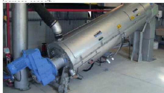
HUBER Screw Press S-PRESS: Specific power consumption < 0.01 kWh/kg DR
