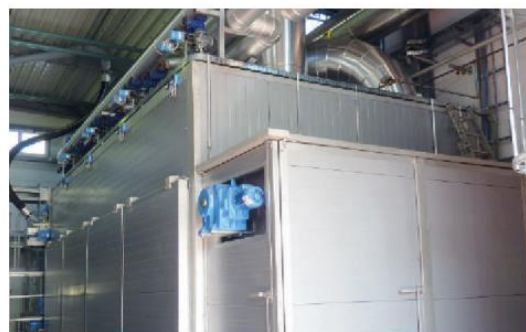
HUBER Belt Dryer BT for sewage sludge drying up to > 90 % DS
