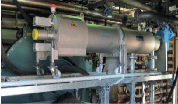
Coarse material separation from fermentation residues at an organic waste fermentation plant
