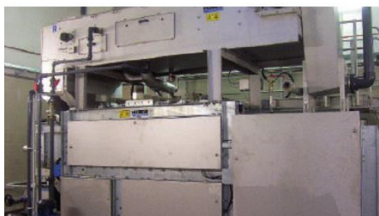
The HUBER Bogenpress B-PRESS can be combined with the HUBER Belt Thickener DrainBelt unit to further
